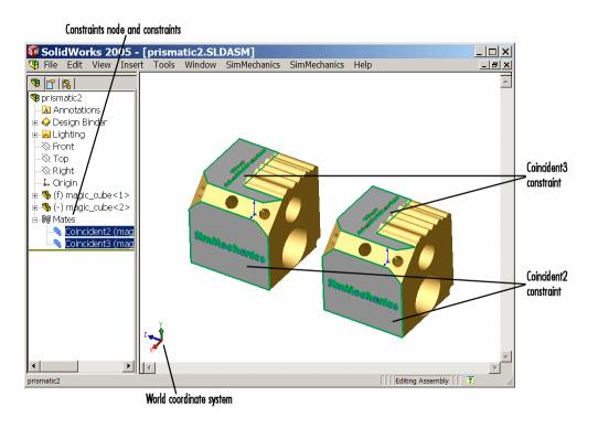
Two Planar Constraints on Two Cubes (SolidWorks)
