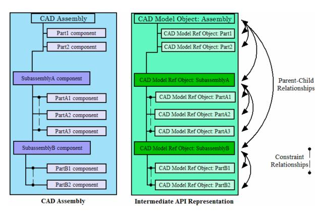
CAD Assembly and Intermediate API Representation: Parallel Hierarchies
